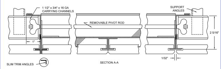
\* Wall or Ceiling opening for KSTC door shall be  $\frac{3}{8}$ " larger than the order size. e.g. for 24"(H) x48"(W) DOOR, opening size shall be 24  $\frac{3}{8}$  x 48  $\frac{3}{8}$ "
